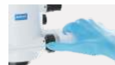
Adjust the fine focus knob
